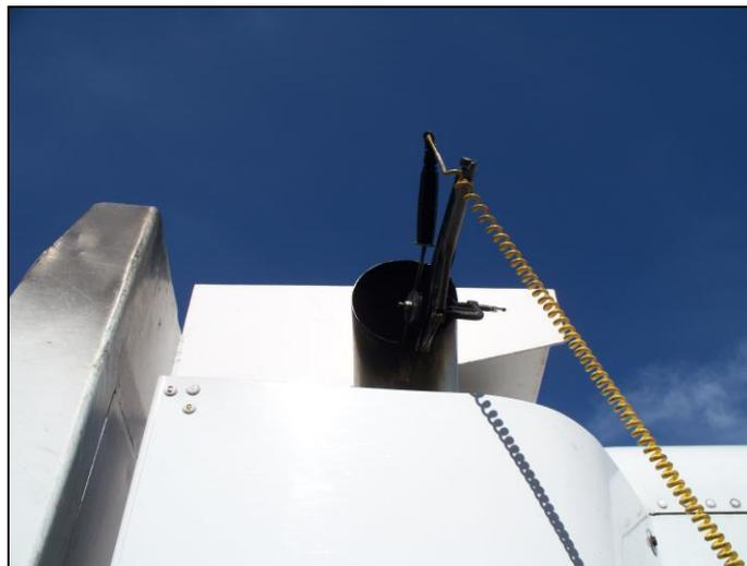
Once the exhaust temperature has stabilized, the test unit has reached its peak operating temperature. Exhaust temperature is critical to the completion of a successful evaluation, since temperature changes identify changes in load and
