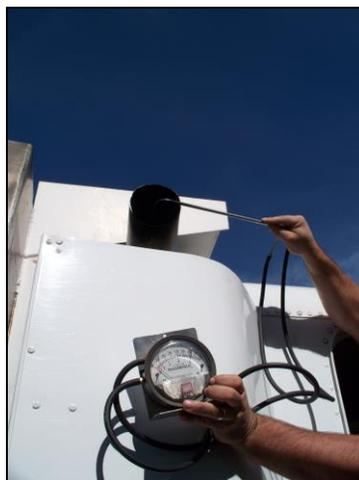
The above photograph shows one method in which exhaust pressure can be monitored during the Carbon Balance test procedure. In this case, exhaust pressure is ascertained through the use of a Magnahelic gauge. This type of stringent regime further documents the inherent accuracy of the Carbon Balance test.
