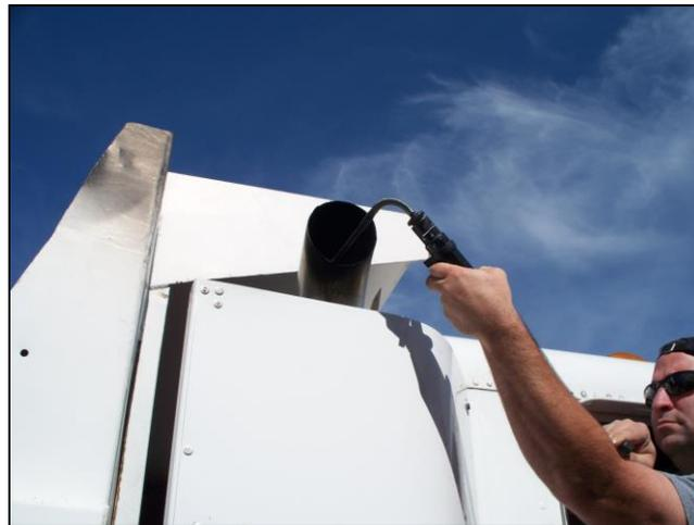
The above photograph demonstrates a typical method in which soot particulate volume is monitored during the Carbon Balance test. This method is the Bacharach Smoke Spot test. It is extremely accurate, portable, and repeatable. It is a valuable tool in smoke spot testing when comparing baseline (untreated) exhaust to catalyst treated exhaust.
