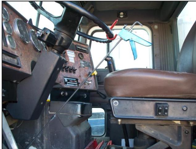
An aftermarket throttle lock is utilized, as one method, to secure engine RPM. This provides a steady state condition in which consistent data can be collected. Should the engine RPM fluctuate erratically and uncontrollably, the test unit would be disqualified from further consideration.
