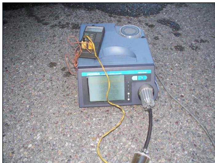
Finally, the data being recorded is collected through a non-dispersive, infrared analyzer. Equipment such as this is EPA approved and CFR 40 rated. This analyzer has a high degree of accuracy, and repeatability. It is central to the Carbon Balance procedure in that it identifies baseline carbon and oxygen levels,
