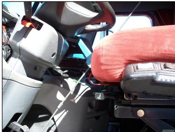
An aftermarket throttle position lock is utilized, as one method, to secure engine RPM. This provides a steady state condition in which consistent data can be collected. Should the engine RPM fluctuate erratically and uncontrollably, the test unit would be disqualified from further consideration.
